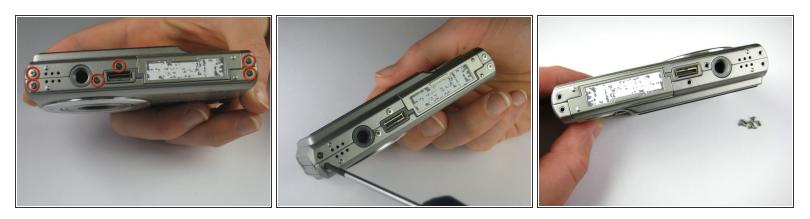
Remove the six Phillips screws (3.69 mm) from the bottom of the camera casing.
