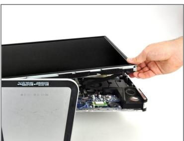
⚠ Lay the iMac down on a table before you remove the LCD so that it doesn't fall.
