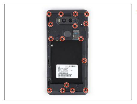
Remove the sixteen 4mm Phillips #00 screws attaching the back cover to the motherboard.
