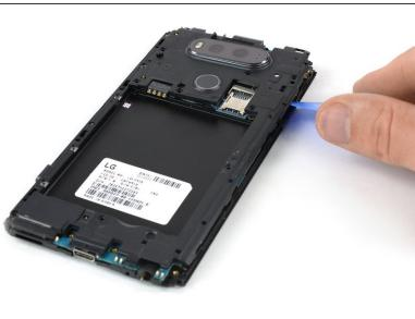
Slide the opening pick along the mid frame and flip it sideways to open the plastic clamps holding the motherboard cover in its place.
