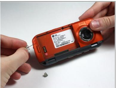
Remove the 5 screw covers on the back of the phone using a Push Pin.
