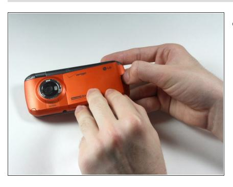
Push/pull the latch away from the camera, causing the battery to pop out.
