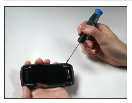
Remove the four 3.44 mm screws that were under the covers using a Phillips #00 Screwdriver.
