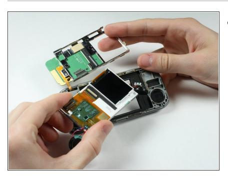
The Number Keypad and its metal casing are attached to the clear plastic screen that the LCD Screen was in. Replace both the Keypad and the casing as a unit.
