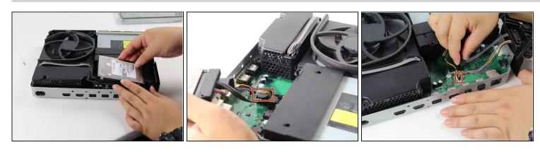
• Gently disconnect the hard drive from the motherboard (at the two plastic connector bodies).
