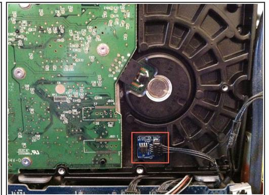
**⚠** A hard drive thermal sensor may be present on some models. If your logic board is missing the hard drive thermal sensor socket highlighted in red in the first picture, skip this step.
