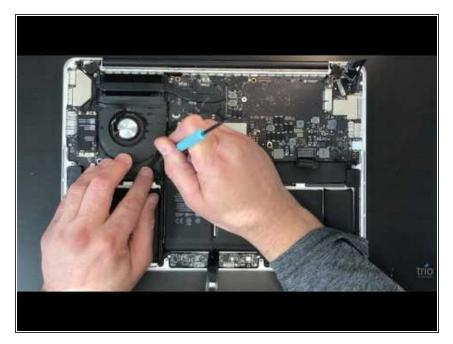
Your first step is to remove your MacBooks main Logic Board, this process will very from model to model and the guides are readily available on iFixit. For this example we will be disassembling an A1502 MacBook Pro w/ Force Touch.
