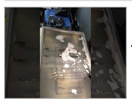
Placing the board in an ultrasonic bath for 15 minutes at 40c with some type of electronics safe detergent will ensure that corrosion that is not visible to the naked eye will be removed. Electricity is the catalyst for corrosion, even a small amount left untreated can come back to bite you. In my opinion a toothbrush and alcohol alone is risky.
