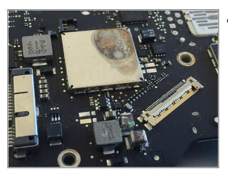
Place the MLB on a lint free towel and begin to carefully remove any visible corrosion with a tooth brush and 99% Isopropyl alcohol. AT this point I would take pictures of the affected areas before cleaning so you have an idea of where to start diagnostics once the board has been cleaned.
