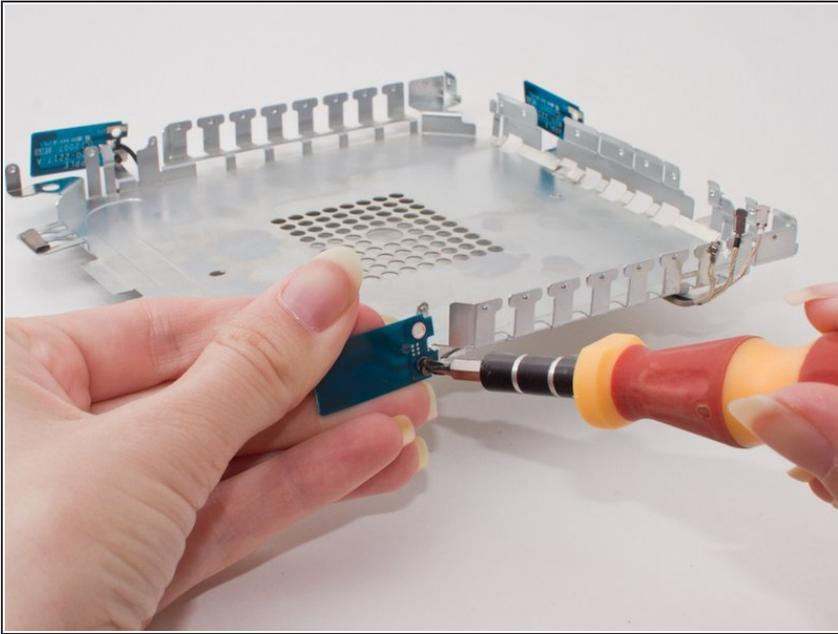
**⚠ Caution:** Be careful not to bend the metal strip that the antenna is attached to. This may cause problems during reassembly and use.
