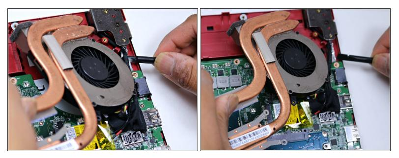
• Continue to use the spudger to carefully separate the wires of the power cord from the laptop.
