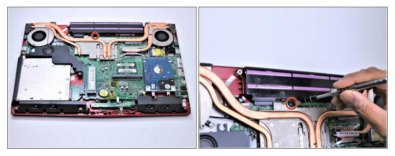
Unscrew the single 5.5mm Phillips #1 screw keeping the battery secure.
