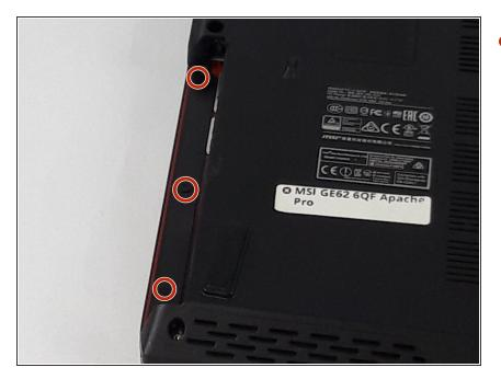
Use a Phillips screwdriver to remove the three screws along the edge of the optical drive bay.
