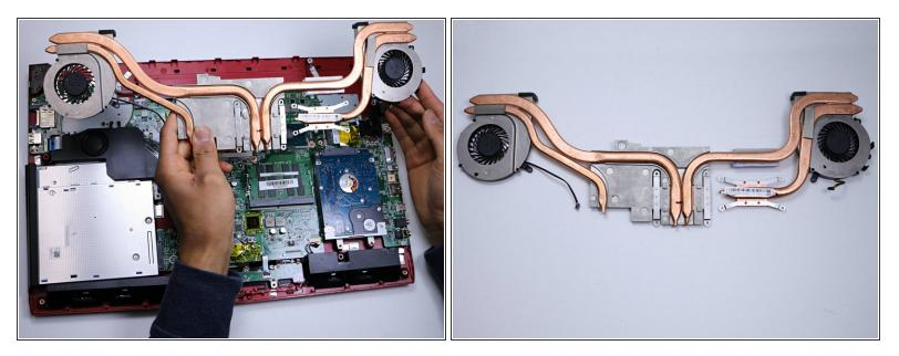
• Fully remove the fans from the rest of the laptop.
