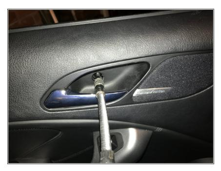
Using a T20 Torx driver with extension, remove all 5 bolts.
