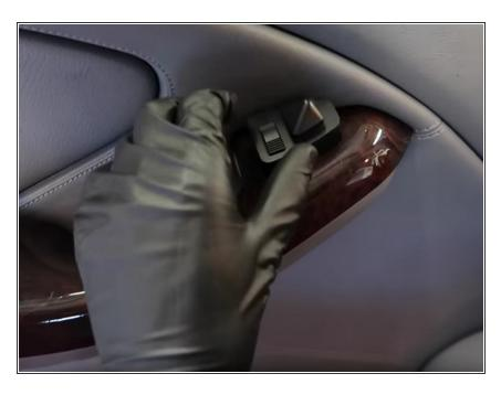
If you're working on the driver side door, remove the mirror control module. Disconnect it from its wiring plug.
