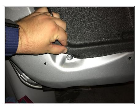
While you're in here, inspect and tighten the bottom bolt.
