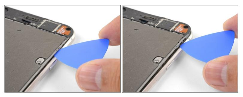
Insert an opening pick into the right edge of the phone and slide it upwards towards the top right clip.
