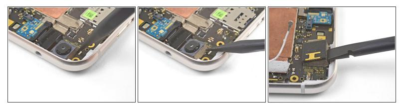
• Use the point of a spudger to pry up and loosen the front facing camera module from its socket.
