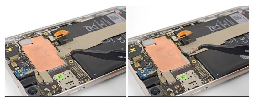
• Use tweezers to peel up the tape at the top of the interconnect cable.
