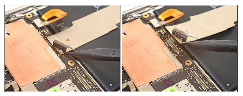
• Use the point of a spudger to pry up and disconnect the interconnect cable from the motherboard.
