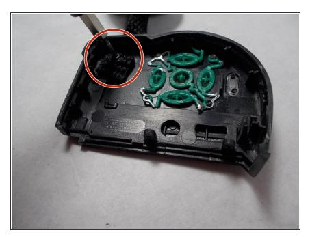
Use your screwdriver to remove the 1 mm Phillips head screw and release the strap.
