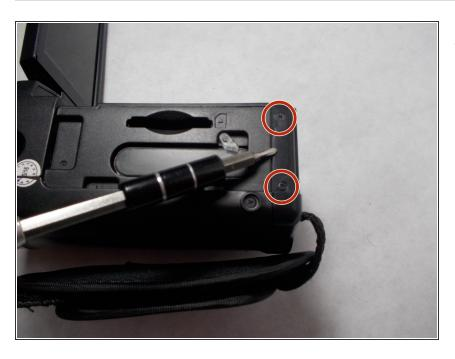
Remove the 1 mm circled screws with the Phillips head #000 screwdriver.
