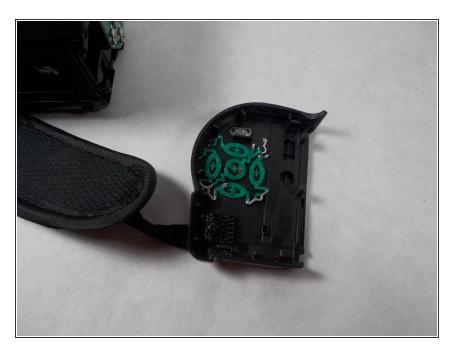
Once all previous screws have been removed the panel can be pulled off of the camera.
