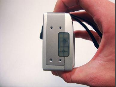
Remove the four 4.7 mm screws on the left side of the camera.
