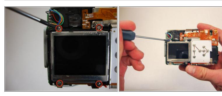
• Using a Phillips #00 remove the four 4.40 mm screws that secure the LCD screen to the frame.
