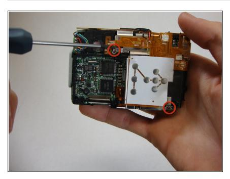
Using a Phillips #00 screwdriver, remove the two screws securing the electric strip casing on the back of the camera.
