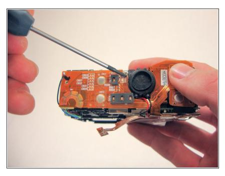
On the top of the camera where the shutter button is located, remove the screws located near the speaker that secure the electric strip casing.
