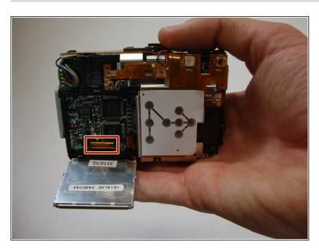
Allow the LCD screen to flip down.
