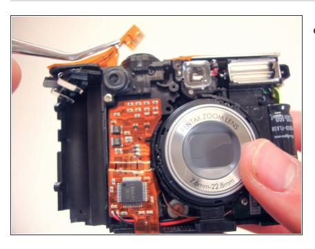
Ensure there are two ends of the electric strip detached from the camera.
