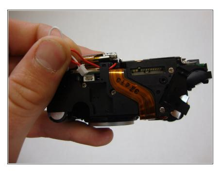
Unplug the connected red and white wires. They will come out with the small white casing.
