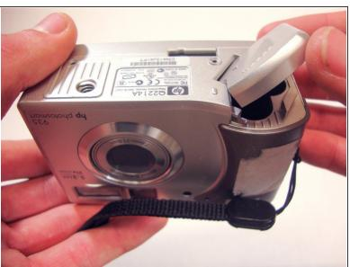
Slide the bottom cover in the direction of the arrow to open it.
