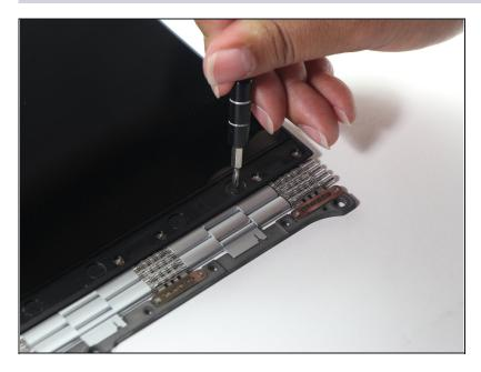
• Remove the eight #0 2.4mm Phillips screws holding down the monitor.
