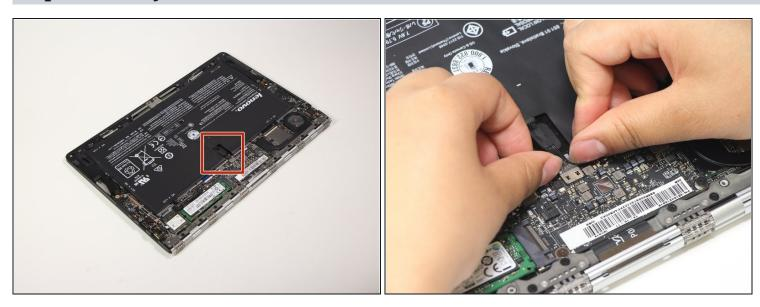
Push the black battery cable towards the battery to disconnect it.
