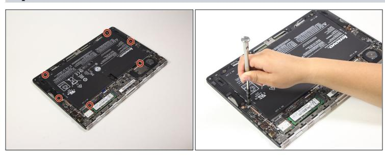
• Remove the six #0 3.8mm Phillips screws from the battery.
