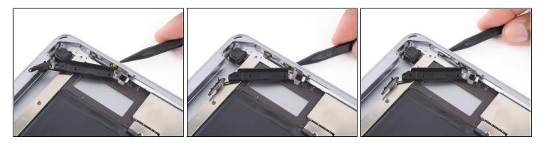
• Use the pointed tip of a spudger to nudge the two volume button covers out of their housing in the rear case.
