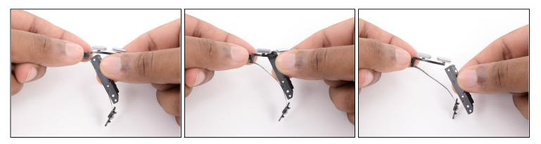
• Gently peel the case buttons' ribbon cable off the metal volume button bracket.
