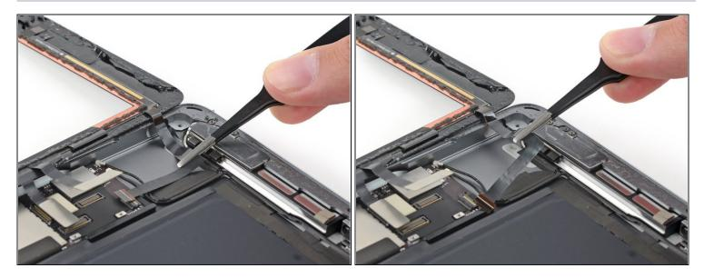
• Carefully peel the home button ribbon cable up off of the adhesive holding it to the rear case.
