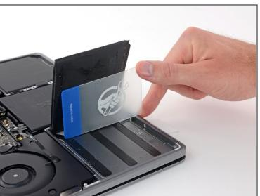
• Twist the card to raise the battery cell until it fully separates from the aluminum case.
