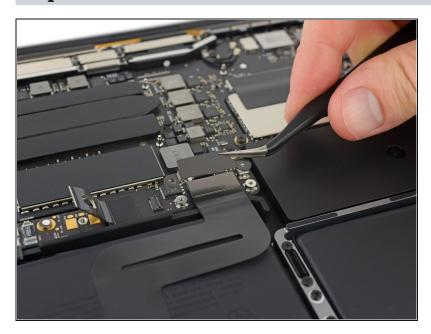
Remove the trackpad cable connector bracket.
