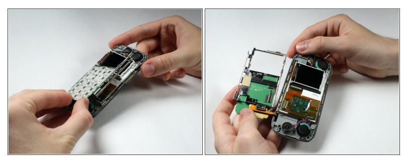
Because the Number Keypad is attached on one side and on top of the outer screen, open its metal casing, in a "door-opening" manner.
