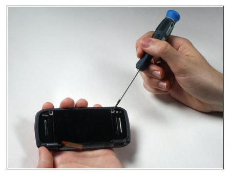
Remove the four 3.44 mm screws that were under the covers using a Phillips #00 Screwdriver.
