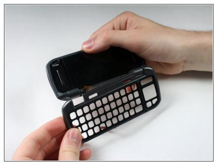
• After removing the circuit board and key board, separate the top part with the screen from the bottom part by detaching the hinges.
