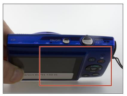
Locate the back plate of the camera (contains the LCD screen and menu buttons).
