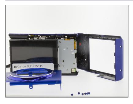
Once the back plate and face plate have been removed, you can begin to remove the LCD screen.
