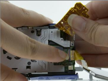
With the screen off to the side, and the horizontal electrical ribbon attached to it out of the way, gently lift the vertical electrical transducer ribbon to expose the salmon colored clip holding the horizontal ribbon in place.
