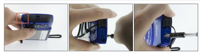
• Remove the next 2 screws located behind the AV port using the same Phillips #00 screwdriver.
