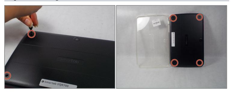
• There are four screws with each one in each corner. Use the screwdriver to unscrew the back or bottom of the device.
