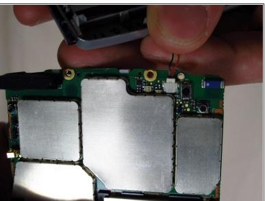
Gently pry the motherboard out of the front casing, bottom first.
