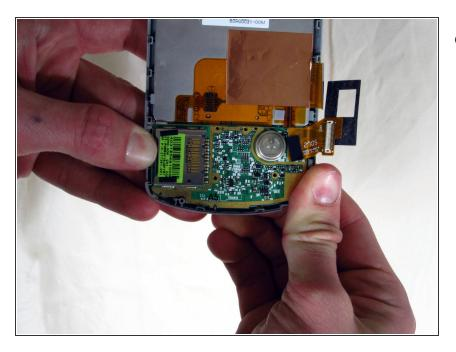
Carefully pop the keyboard out by bending the phone casing to free the keyboard from the casing.
