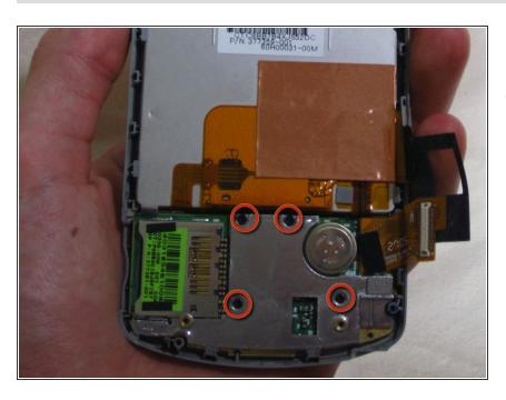
Unscrew the four small screws holding the keyboard in place using a 00 Phillips screwdriver.
