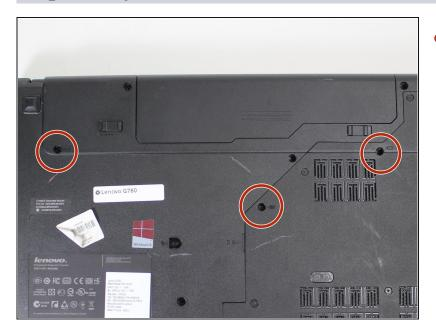
Remove the three 9mm keyboard screws with a #0 Phillips screwdriver.
