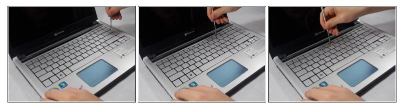
Use the small metal spudger to push in each of the clips on the keyboard
