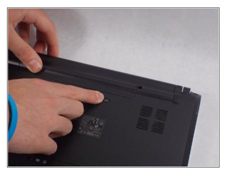
Locate the switch that releases the battery and slide it to the right.
