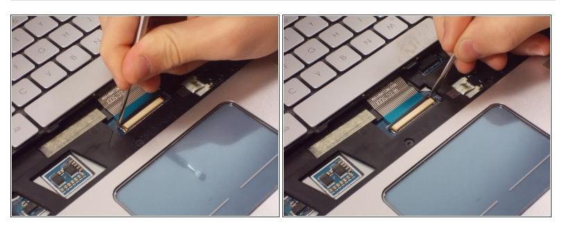
Use the small spudger to slide the cable lock up on both sides of the connector and slide the cable out
