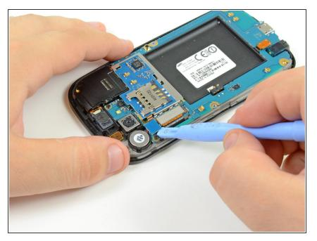
Use the flat edge of a plastic opening tool to pry the SIM Board connector off its socket on the motherboard.
