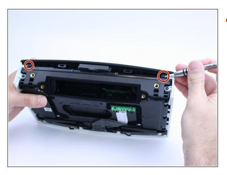
Remove the two screws holding the speaker grille in place.
