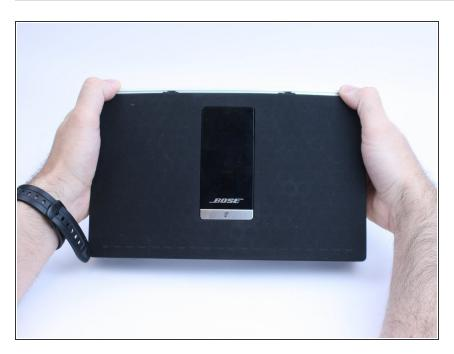
Grip the sides of the device and push the speaker grille down and out.
