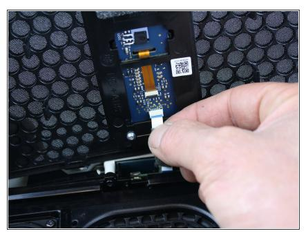
• Gently release the ribbon from its connector and remove the grille.
