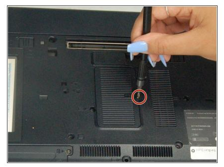
Use a screwdriver to remove the single screw on the covering located on the back of the laptop.
