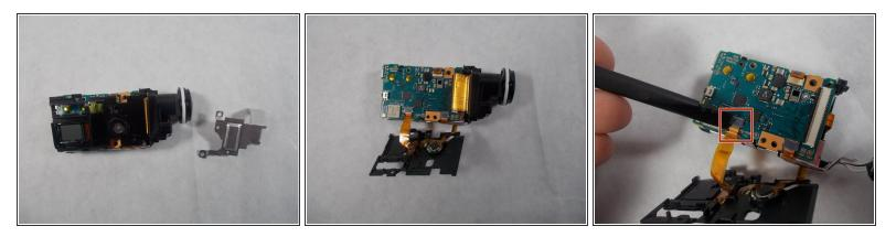
• Remove the screws connected to the silver metal plate, once done, remove the plate by pulling the back up and pushing it towards the front. Now remove the screw directly above the LCD display, this will loosen the plastic up. Pull the plastic up gently, it will be connected by cables on the bottom. From here remove the speaker.
