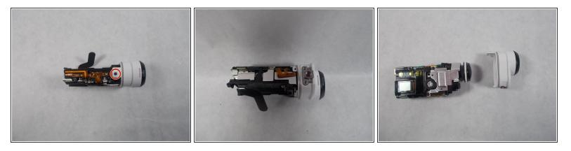
• You'll see a screw on the top of the device, towards the front, remove this screw. Next pull the tabs on the bottom and top of the lens, and pull outward, this will remove the lens housing from the body. Once removed, flip the device onto its side, leaving the LCD display facing up.
