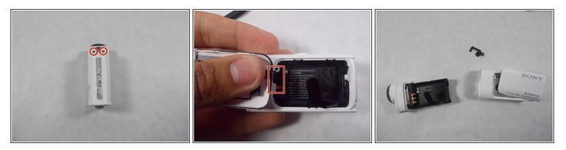
• Start by removing the two screws on the bottom, and the screw inside the battery room. Once these are removed, slide the door out, and the small piece of plastic with the door. Now, grab the lens and pull the body out of the plastic, this will reveal the insides of the device.
