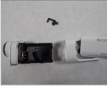
• Start by removing the two screws on the bottom, and the screw inside the battery room. Once these are removed, slide the door out, and the small piece of plastic with the door. Now, grab the lens and pull the body out of the plastic, this will reveal the insides of the device.
