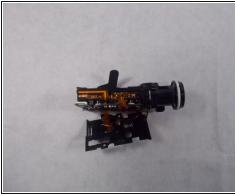
Remove the screws connected to the silver metal plate, once done, remove the plate by pulling
