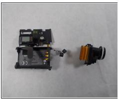
• This will reveal the thick cable, carefully pull this cable towards the front. Next remove one last screw on the top of the device, and slowly pull the lens out. You'll notice that the microphone is still connected to the lens, just pop these out and the lens is off.
