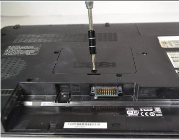
• Use a J00 bit to unscrew the single 4mm screw that leads to the RAM Memory compartment.
