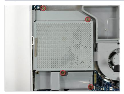
Remove the four 7 mm Phillips screws securing the optical drive to the midplane.
