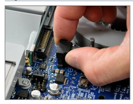
Disconnect the SATA data cable by pulling its connector straight up off the logic board.
