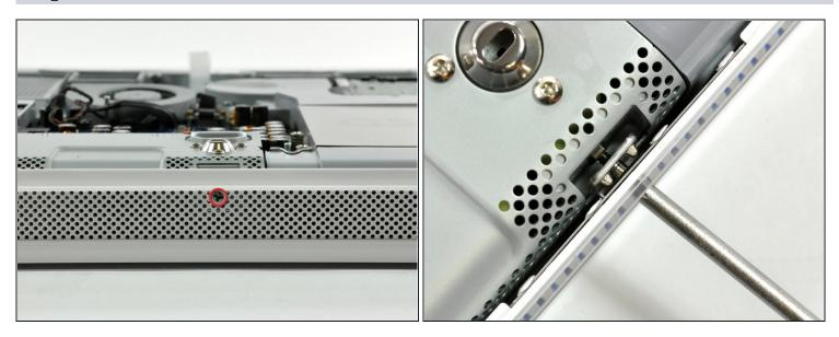
• Rotate the center Phillips screw on the bottom of the iMac clockwise until the rear panel clamp contacts the edge of the case.
