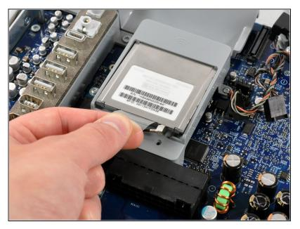
Lift the AirPort card slightly by its plastic tab and pull it straight away from its socket.
