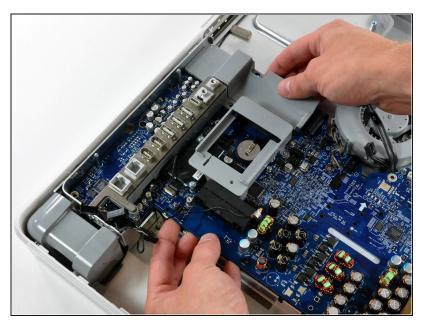
Gently lift the logic board from its left side to clear the two pins mounted to the midplane.
