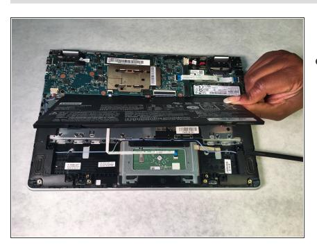
Remove the battery carefully from the device by lifting up the edge nearest you and then gently pull toward you to disconnect the power wires. To reassemble your device, follow these instructions in reverse order.
