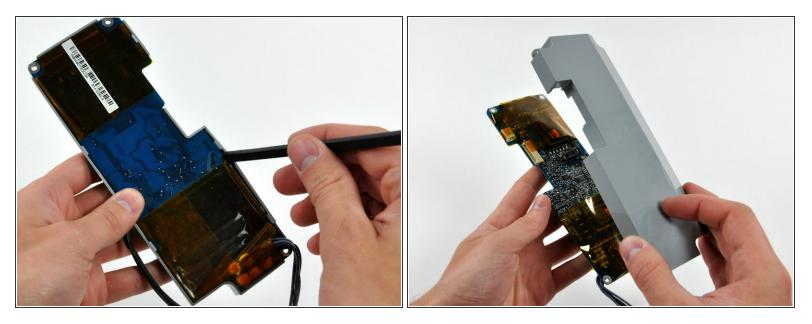
F If you wish to replace just the inverter board, use a spudger to pry off its plastic cover.
