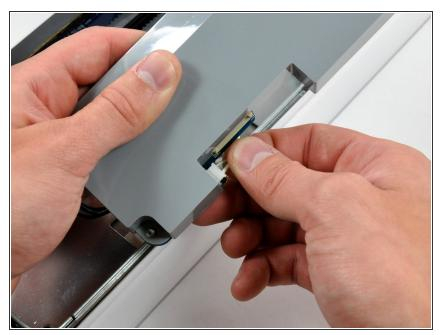
• Disconnect the small inverter cable connector by pulling it straight away from its socket.
