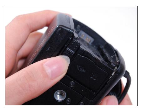
Locate the slider labeled "BATT" and pull it back from the battery with your thumb.
