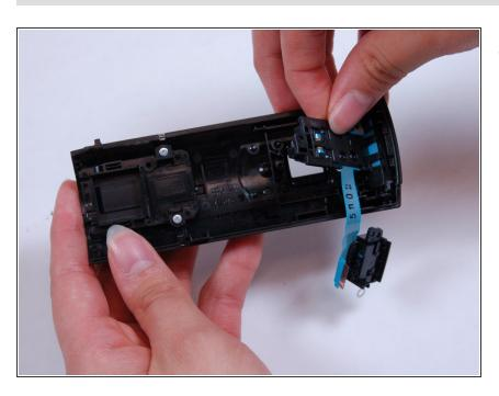
You are now free to remove the recording button, as well as its connection strip.
