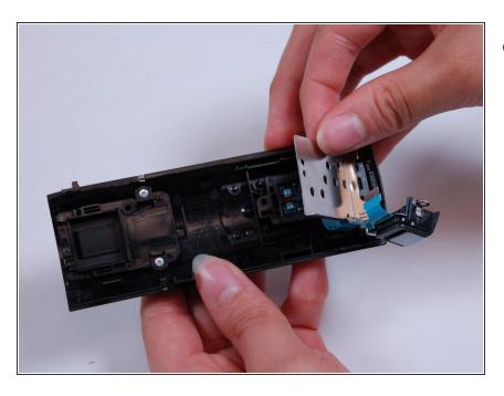
Carefully remove the metal frame from the top casing.
