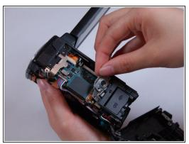
Carefully remove the bottom casing with your fingers.
