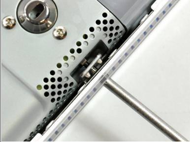
Rotate the center Phillips screw on the bottom of the iMac clockwise until the rear panel clamp contacts the edge of the case.
