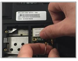
Unplug the two connecting cables by lifting them up. They should unclip easily.
