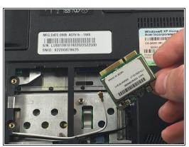
Remove the screw Phillips #0 (M2-L3 mm) holding down the network card. Pull out the card.
