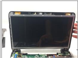
Separate the upper casing from the display.
