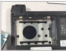
Remove the hard drive by sliding it to the left and pull it out.
