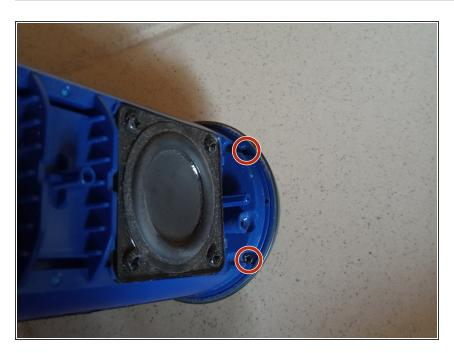
loosen the screws to remove the outer frame
