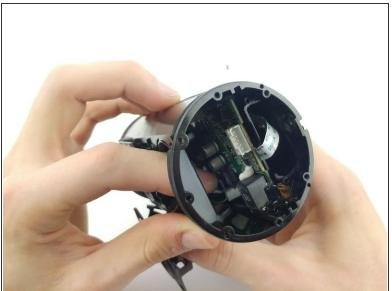
Remove the 3 pin connector from the USB chip.
