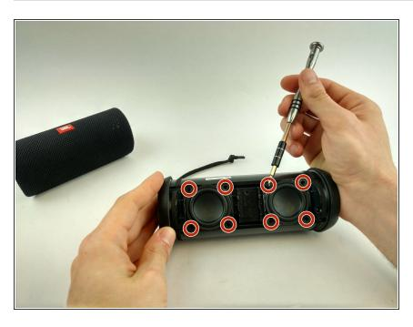
Remove the 8 8.9mm Phillips #00 screws to unfasten the side passive drivers. Set the screws and side passive drivers aside safely.
