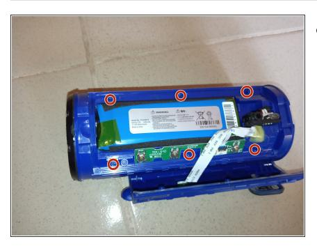
remove screws to expose usb port
