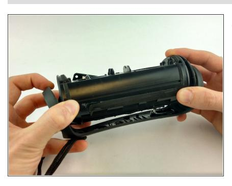
Carefully remove outer frame to expose the inner components of the speaker.
