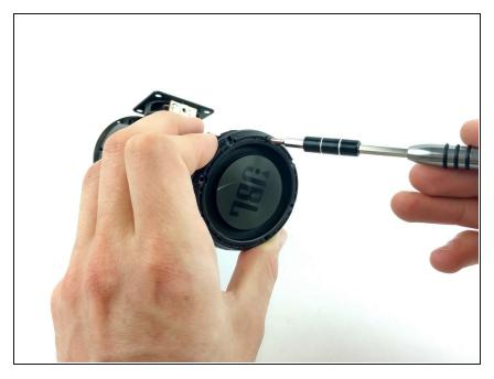
Remove the 7 8.9mm Phillips #00 screws fastening the two side passive drivers. Then remove the side passive drivers themselves. Be sure to set them somewhere safe to ensure they aren't lost.
