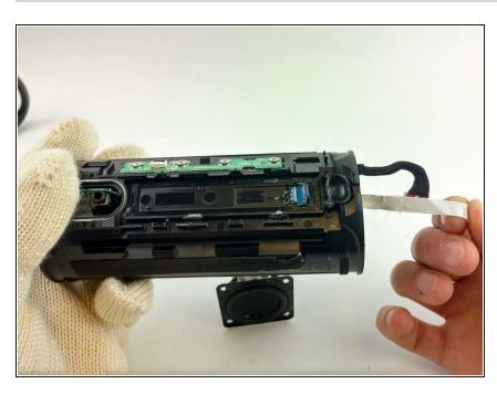
Remove the ribbon holding the battery. When the ribbon is gently pulled until fully removed from the inner housing, the battery will be unfastened and removable. To reassemble your device, follow these instructions in reverse order.
