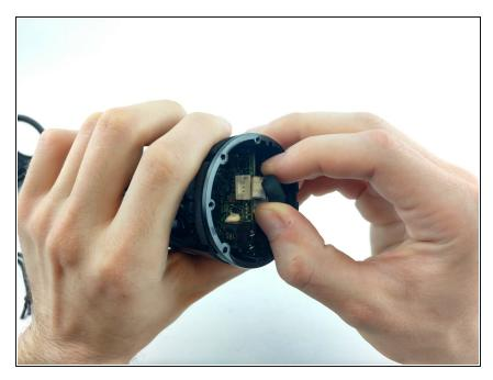
Carefully remove the 5 pin connector from motherboard using your hands
