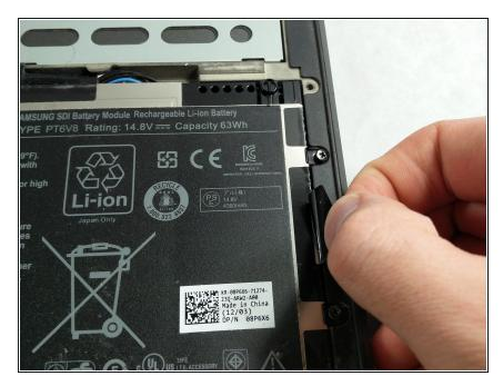
After removing the two screws, gently lift up the battery with the small plastic tab attached.
