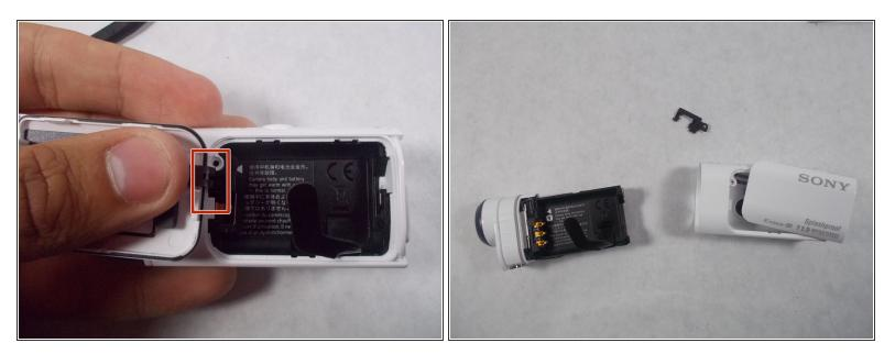
• Pull out the small plastic bracket that holds the door in place.
