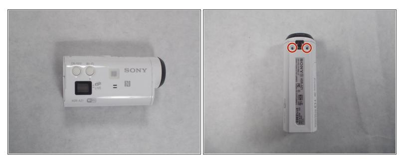
• Remove the screws on the bottom of the device.
