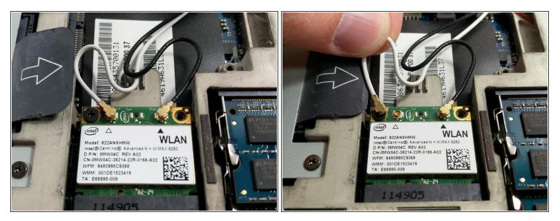
(i) Your Wi-Fi card will have two coaxial cable wires connected to it.
