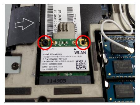
Once the wires are removed, use an appropriate screwdriver to remove the screws holding down the Wi-Fi card.
