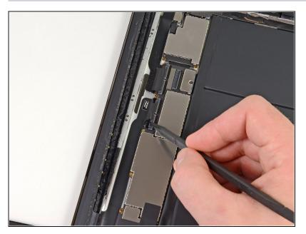
• Using the tip of a spudger, peel back the piece of tape that secures the touchscreen ribbon cable to the logic board.
