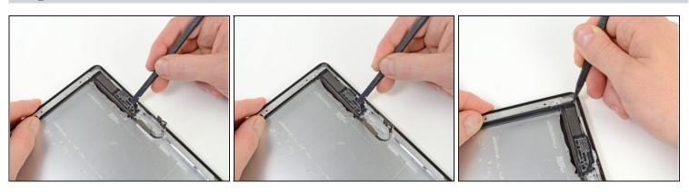
• Using a spudger, carefully push the speaker assembly out of its recess in the aluminum frame.
