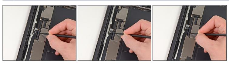
• Flip up the retaining flap on *both* of the touchscreen ribbon cable ZIF connectors.
