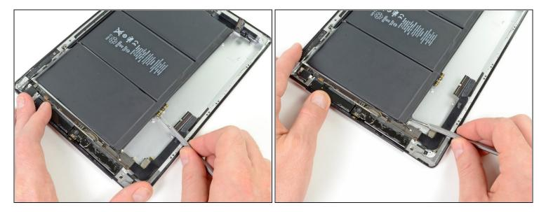
• Continue releasing the adhesive near the top of the battery.
