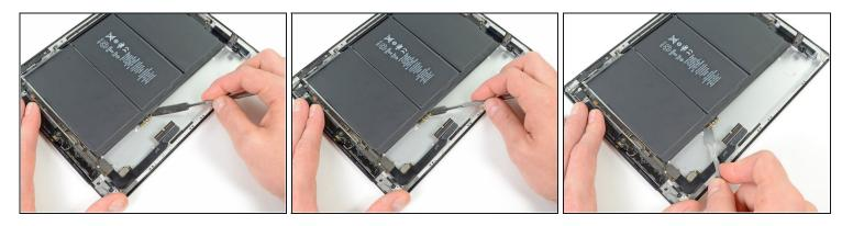
• Carefully slide the metal spudger underneath the battery connector, releasing the adhesive securing it in place.
