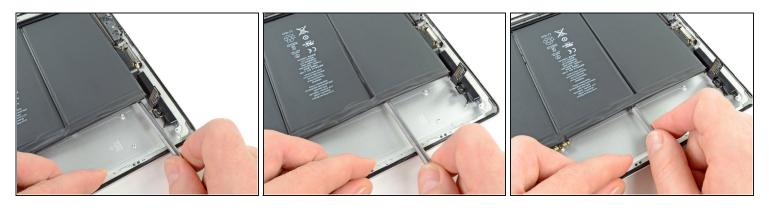
• Starting where the last pass left off, insert the metal spudger another two inches underneath the battery.
