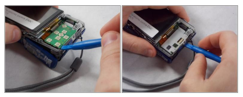
Access the ribbon cables by removing the green button receiver panel using a plastic opening tool. There is a white panel beneath. Carefully remove this using a plastic opening tool. The white panel may require some elbow grease to get it off, and the panel may make a snapping sound as it comes off.
