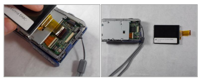
• One of the ribbon cables will be housed behind the screen and the other will be under the panels. Gently pull each free from the housing and remove the screen.
