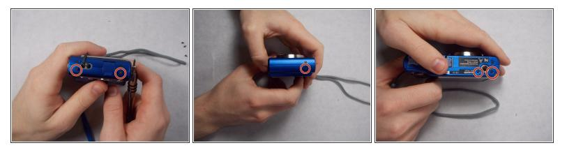
• Remove 5 screws attached to the back case using a 00 Phillips head screwdriver.
