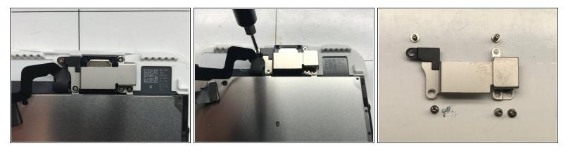
• Remove the five screws holding the earpiece speaker retaining plate in place. These are #000 phillips head screws.
