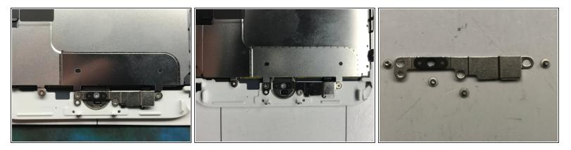
Using your #000 tri-tip screwdriver remove the four screws holding the home button backplate in place.
