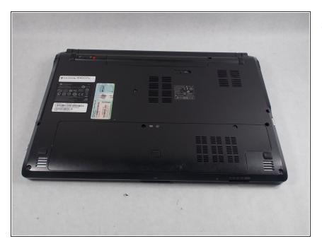
Turn the laptop over so the bottom of the device is facing upwards with the hinge facing away from you.
