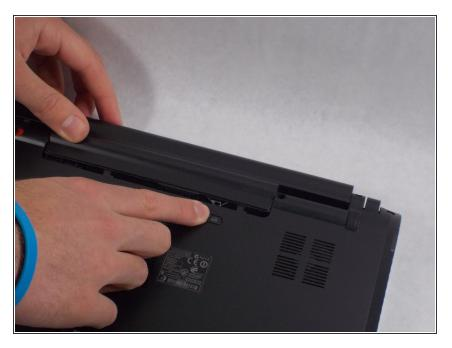
While holding the release switch to the right, pull the battery away from you.
