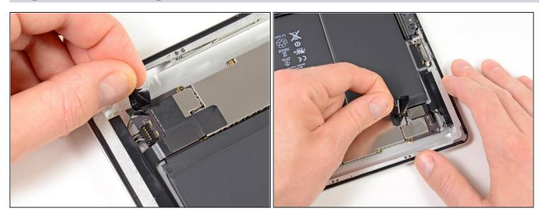
(i) If present, remove the pieces of electrical tape covering the Wi-Fi antenna, speaker cable, and dock connector cable.
