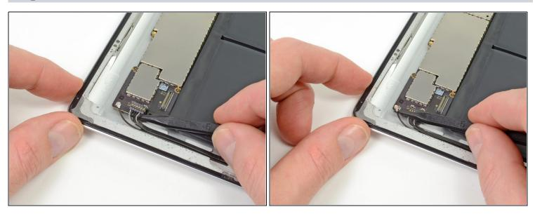
• Use the tip of a spudger to pry the speaker and Wi-Fi antenna connectors straight up off their sockets on the logic board.
