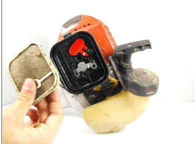
Remove the air filter by gently pulling it away from the unit.
