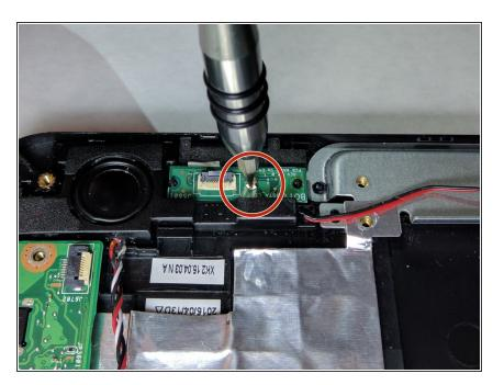
Unscrew the 1 JIS 2mm screw with the J0 bit.
