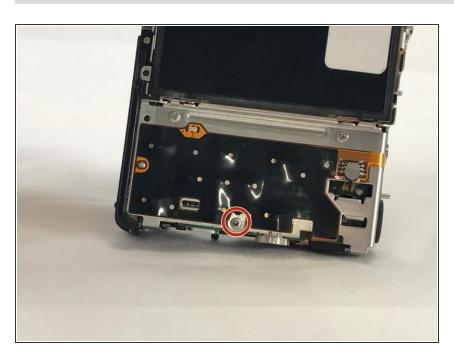
Use a Phillips #000 screwdriver to unscrew the 4mm screw.
