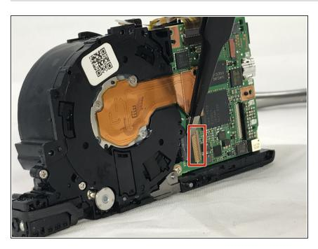
Unplug the ZIF connection between the lens to the main processor.
