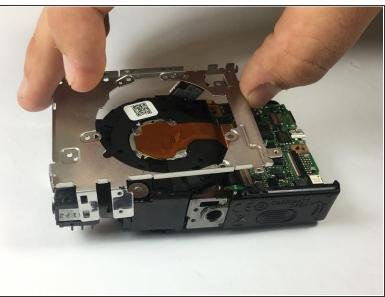
Gently remove the frame. (Make sure to have a firm hold on the rest of the camera at this point)
