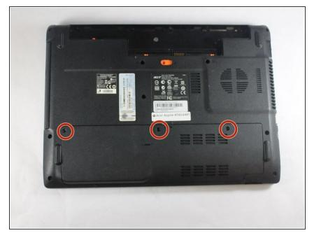
Remove three 7.0 mm screws with a Phillips head screwdriver from the back panel to gain access to the RAM cards.
